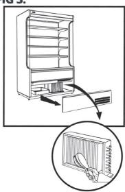
Brush fins vertically with a stiff brush, taking care not to damage them or to push dirt / dust further in, and then vacuum away.
